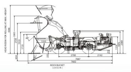
The manufacturer reserves the right to amend/modify the specifications and/or design of this machine at any time without notice. The dimensions are in mm & of standard machine not fitted with any optional items.
